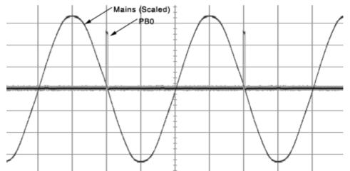
Figure 4. Screenshoot from Oscilloscope, Mains Input and PB0 Output
