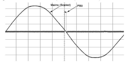
Figure 5. Screenshot from Oscilloscope, Mains Input and PB0 Output
